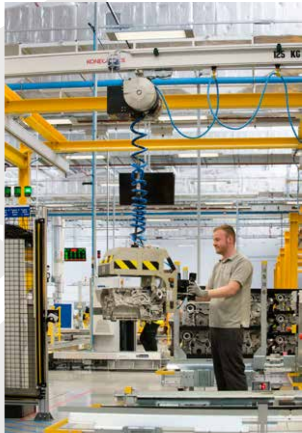
▲ Some 70 Konecranes XMP pillar jib cranes equipped with the popular and versatile CLX electric chain hoist are featured across the JLR site, providing a maximum lifting capacity of 250kg.
